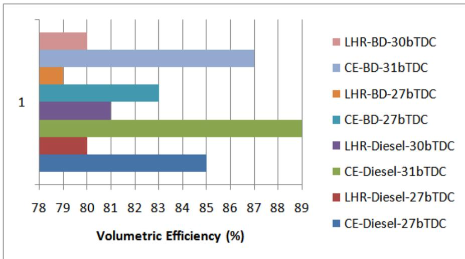
**Figure.8** Bar charts showing the variation of volumetric efficiency at full load operation with test fuels at recommended and optimized injection timings at an injector opening pressure of 190 bar in conventional engine and LHR combustion chamber.
