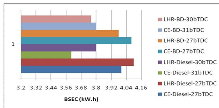
**Figure.5** Bar charts showing the variation of brake specific energy consumption (BSEC) at full load operation with test fuels at recommended and optimized injection timings at an injector opening pressure of 190 bar in CE and LHR combustion chamber.
