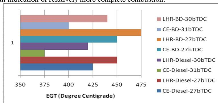
**Figure.6.** Bar charts showing the variation of exhaust gas temperature (EGT) at full load operation with test fuels at recommended and optimized injection timings at an injector opening pressure of 190 bar in conventional engine and LHR combustion chamber.
