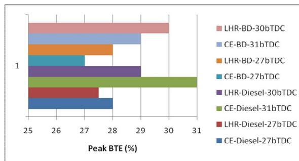
**Figure.4** Bar charts showing the variation of peak brake thermal efficiency (BTE) with test fuels at recommended and optimized injection timings at an injector opening pressure of 190 bar in conventional engine and ceramic coated LHR combustion chamber
