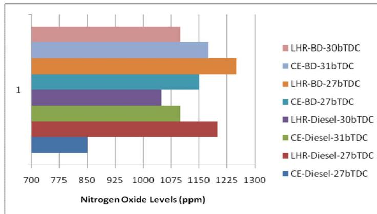
**Figure.10.** Variation of nitrogen oxide levels with brake mean effective pressure (BMEP) in conventional engine (CE) and engine with LHR combustion chamber at recommended injection timing and optimum injection timing and at an injector opening pressure of 190 bar with biodiesel
