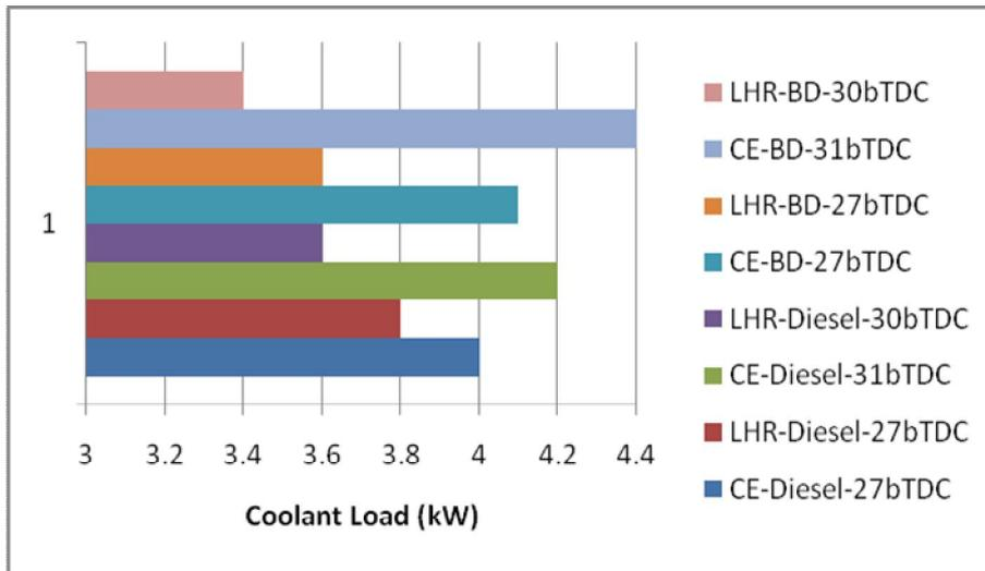
**Figure.7** Bar charts showing the variation of coolant load at full load operation with test fuels at recommended and optimized injection timings at an injector opening pressure of 190 bar in conventional engine and LHR combustion chamber.
