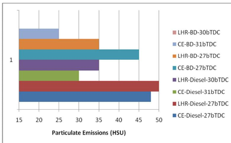
**Figure.9.** Variation of particulate emissions in Hartridge smoke unit (HSU) with brake mean effective pressure (BMEP) in conventional engine (CE) and engine with LHR combustion chamber at recommended injection timing and optimum injection timing and at an injector opening pressure of 190 bar with biodiesel
