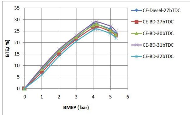
**Figure.2** Variation of brake thermal efficiency (BTE) with brake mean effective pressure (BMEP) in conventional engine (CE) and with various injection timings at an injector opening pressure of 190 bar with biodiesel
