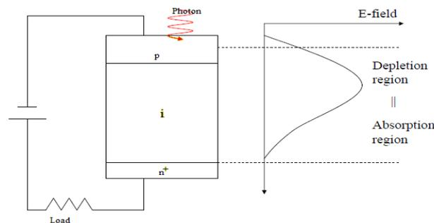
**Fig.2.** PIN photodiode showing combined absorption and depletion
