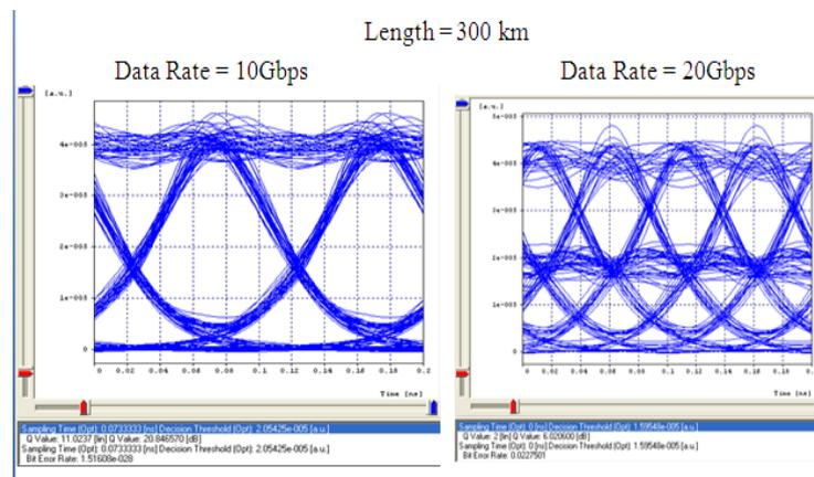
**Fig.6 (c).** Eye pattern for the length of fiber =300km
