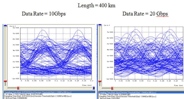
**Fig.6 (d).** Eye pattern for the length of fiber = 400km
