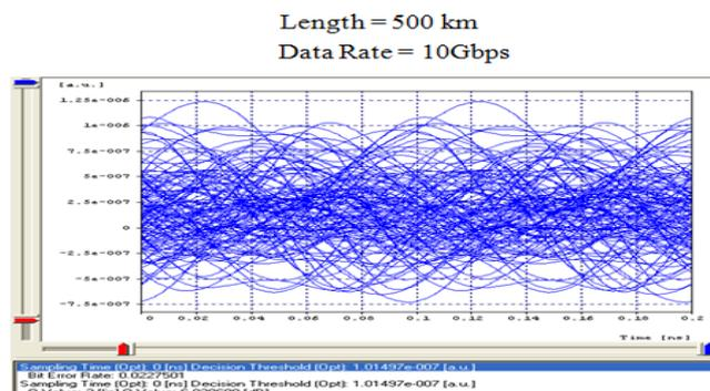
**Fig.6 (e).** Eye pattern for the length of fiber = 500km
