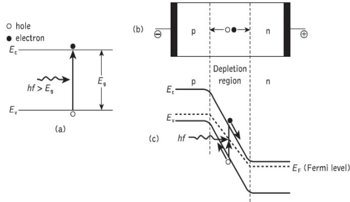
**Fig.1.** Operation of the p-n photodiode
