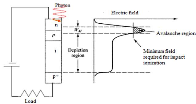
**Fig.3.** Avalanche photodiode showing high electric field region
