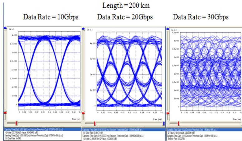
**Fig.6 (b).** Eye pattern for the length of fiber =200km
