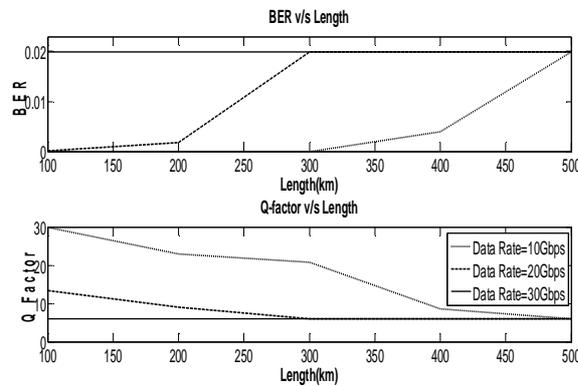
**Fig.7.** BER v/s Length and Q-factor v/s Length
