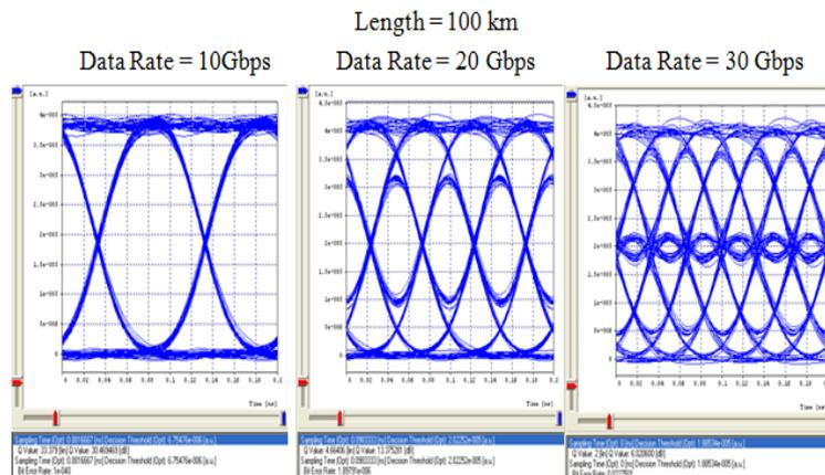
**Fig.6 (a).** Eye pattern for the length of fiber = 100km
