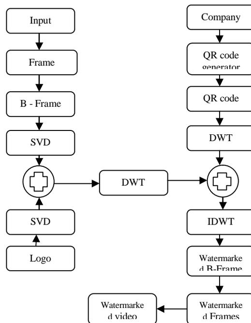
**Figure 5** Block diagram of embedding process
