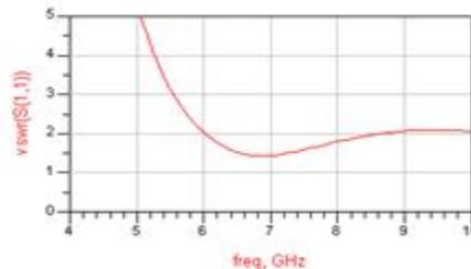
**Fig 5.** VSWR graph for 8,5mm Basic square antenna.
