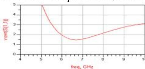
**Fig 6.** VSWR graph for 8,5mm square antenna with bevel.
