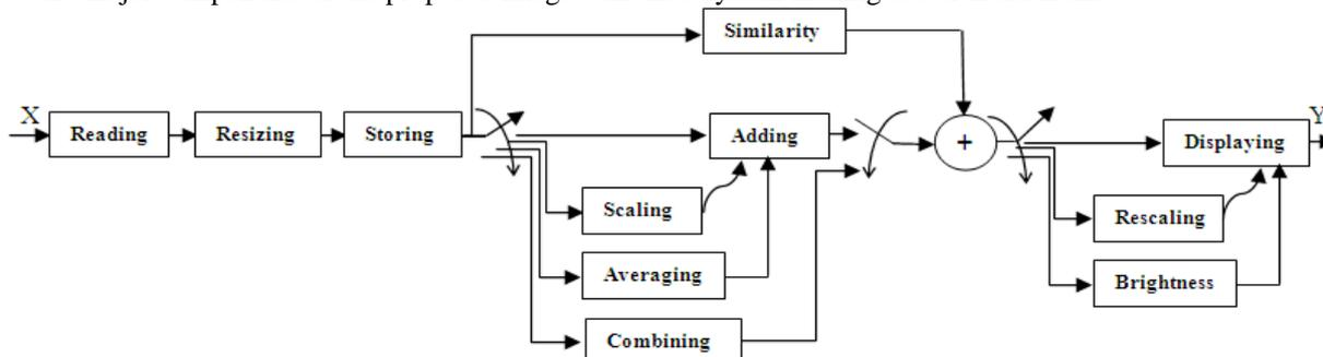
Figure 5 Multi-frame image display system
