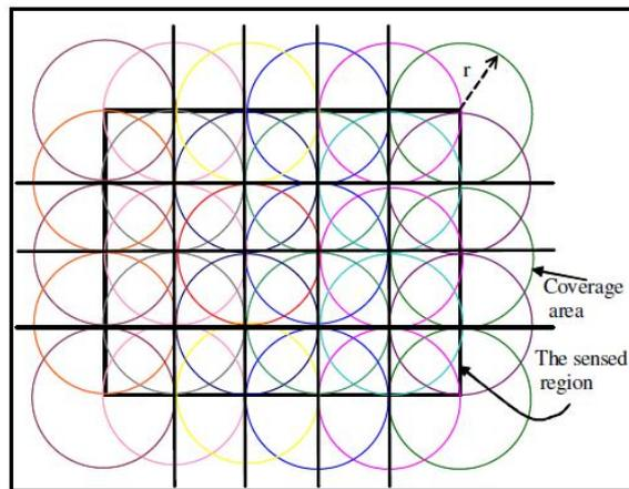
**Figure 1** The model used in equations derivation for the sensed area
