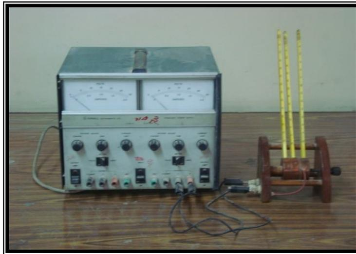
**Figure (8):** Thermal Conductivity Test Instrument
