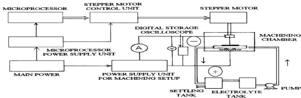
Fig. 1. Various system components of the EMM setup.
