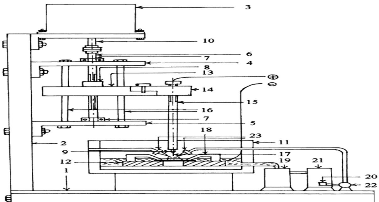
The tool holder to support the main driving screw [6] with the help of two bearings [7]. The main driving screw is passed through the nut [8], which actually holds the tool holding block [9]. The screw rod is keyed with the stepper
