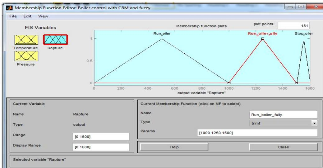
Figure 9 Membership function for the boiler
