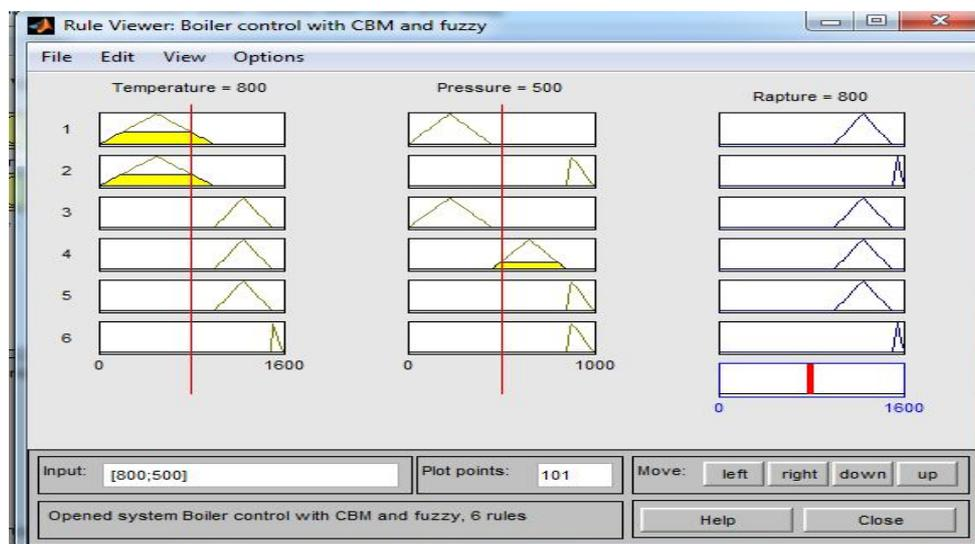
Figure 11 Rule viewer for the boiler
