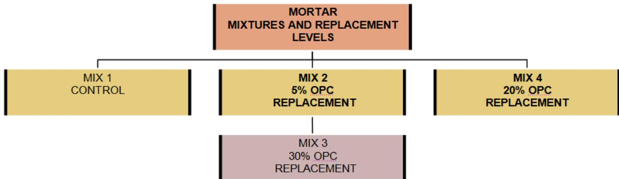
**Figure 1** Experimental mortar mixtures
