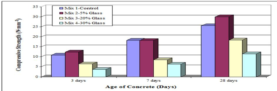
**Figure 3** Compressive strength of waste glass mortar mixes
