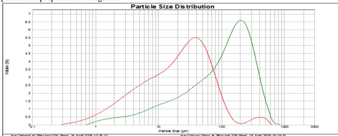
**Figure 2** Particle size distribution for cement and ground glass
