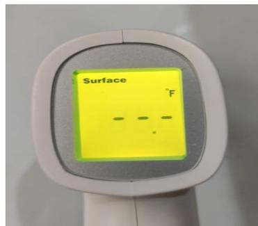
**Figure 2:** An infrared temperature measurement gun set on Surface with Fahrenheit Mode
