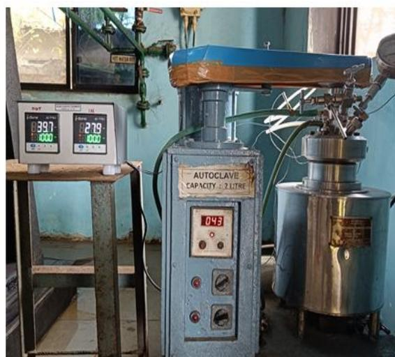
Figure 1:- Autoclave Setup
