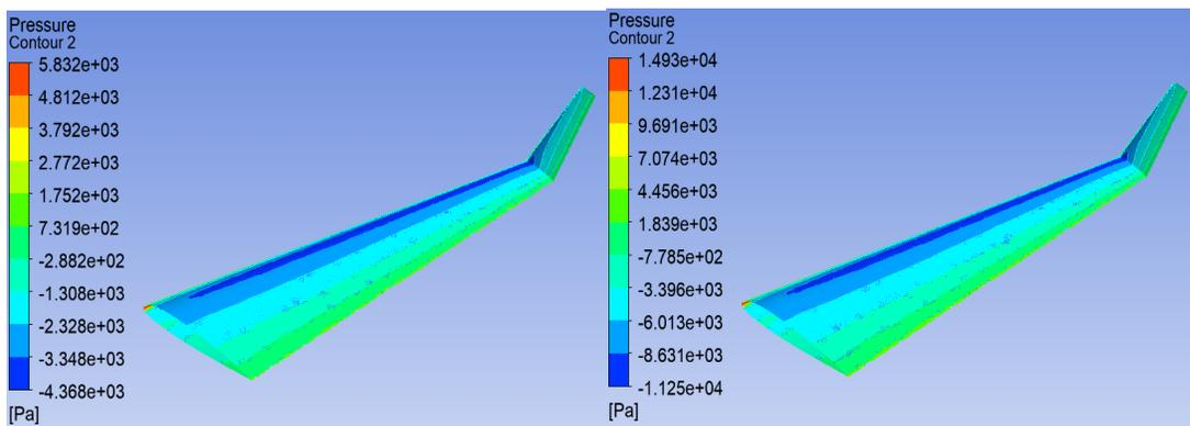
**Figure 9** Pressure contour of wing at 45 degrees cant angle at 100 and 160 m/s
