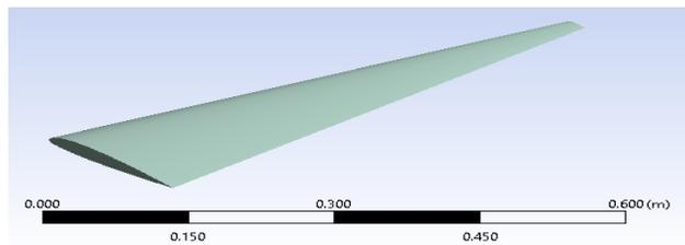
Figure 2 Winglet at 0 degrees
