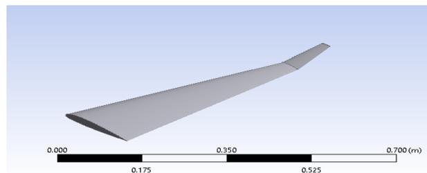
Figure 3 Winglet at 20 degrees
