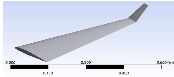
**Figure 4** Winglet at 45 degrees
