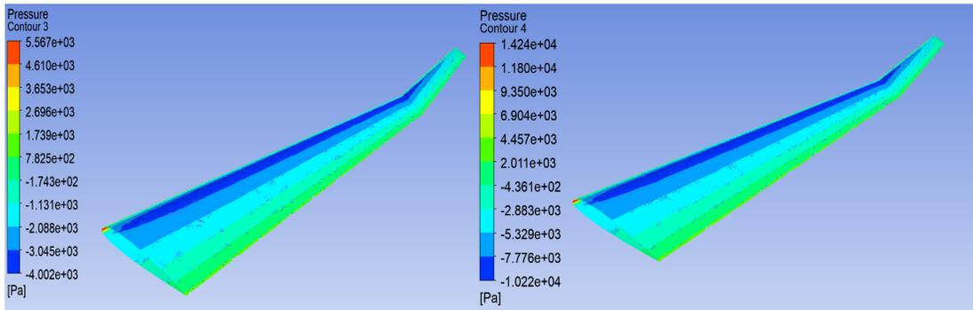
**Figure 8** Pressure contour of wing at 20 degrees cant angle at 100 and 160 m/s
