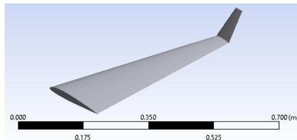
**Figure 5** Winglet at 60 degrees
