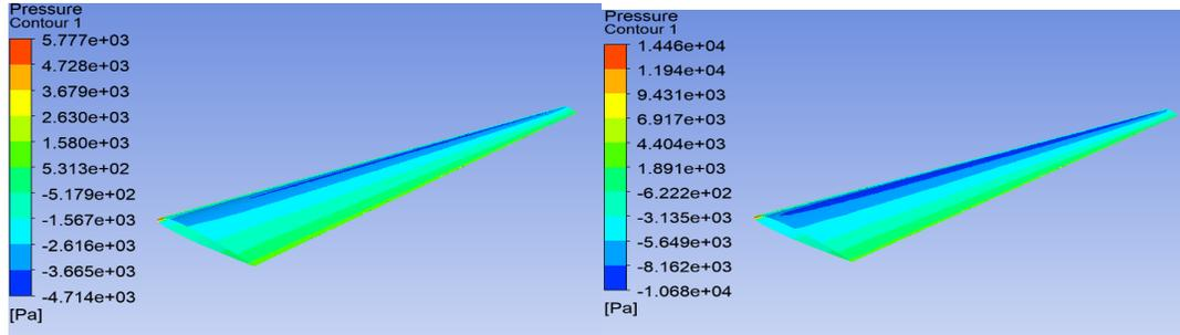
**Figure 7** Pressure contour of wing at 0 degrees cant angle at 100 and 160 m/s
