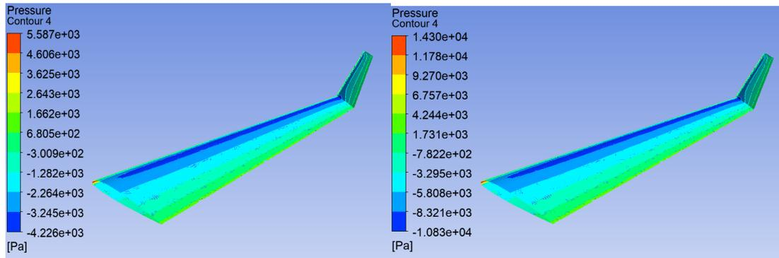
**Figure 10** Pressure contour of wing at 60 degrees cant angle at 100 and 160 m/s
