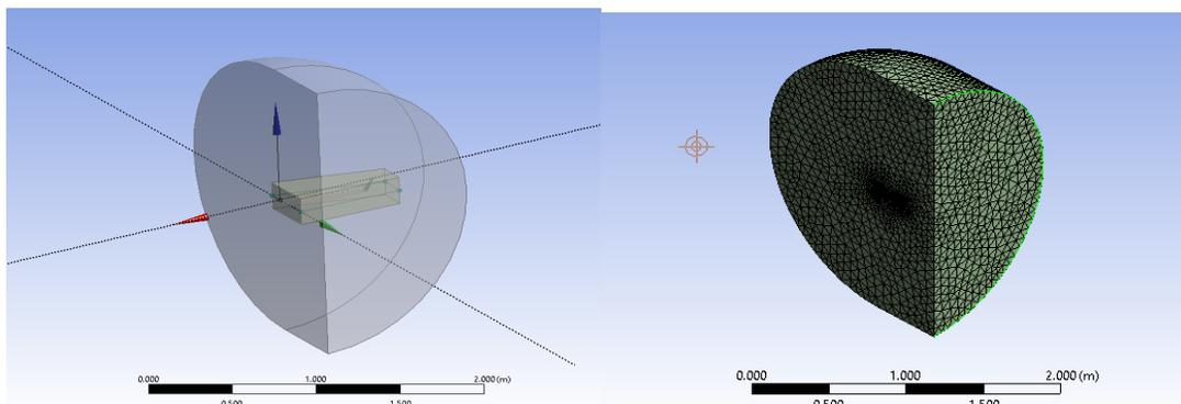
**Figure 6** Control volume and meshing
