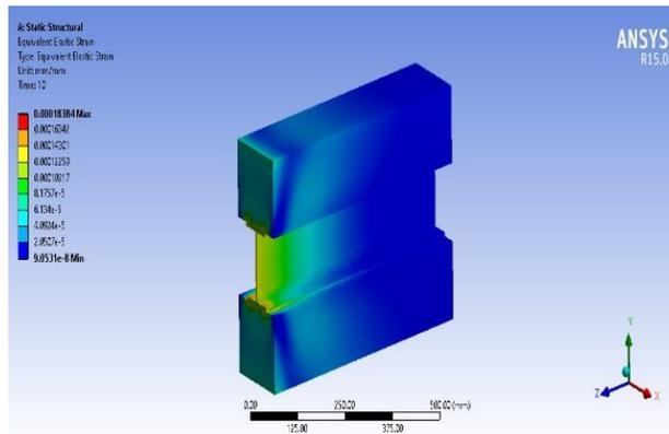
**Figure 7** Stud connector - strain Safety Factor
