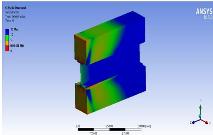
Figure 20 Channel connector – safety factor
