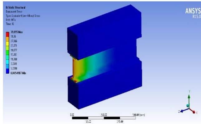
**Figure 12** Channel connector - stress
