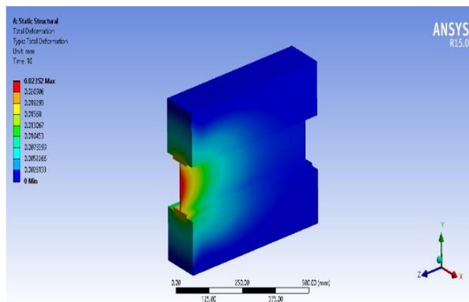
**Figure 5** Stud connector - deformation Stress
