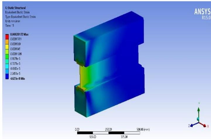
**Figure 19** Channel connector – strain
