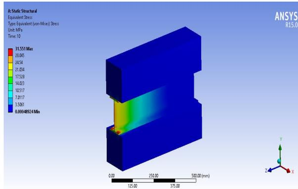
**Figure 6** Stud connector – stress strain
