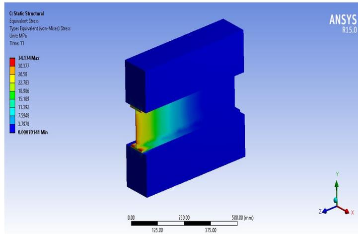
**Figure 18** Channel connector – stress
