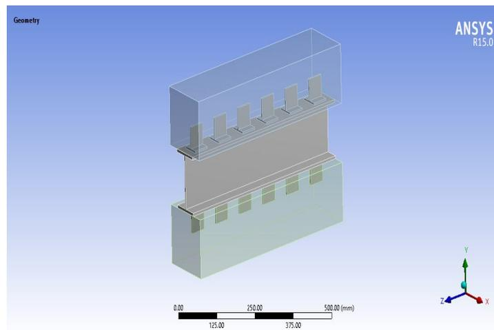
**Figure 15** Tee connector model Mesh
