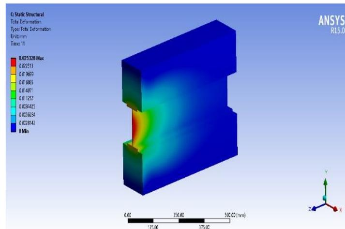
**Figure 17** Channel connector – deformation
