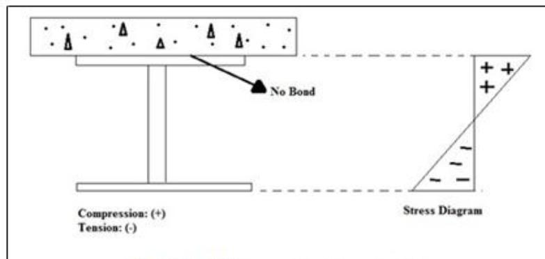
**Figure 1** Steel Joist Supporting Concrete Slab
