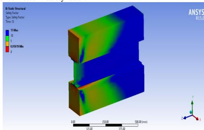
**Figure 14** Channel connector – safety factor
