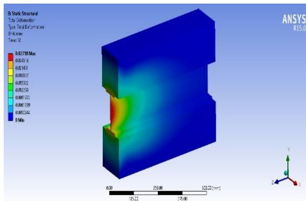
**Figure 11** Channel connector - deformation
