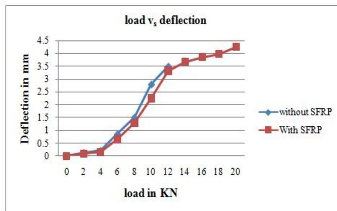
**Figure 8** Cyclic load graphs for T section
