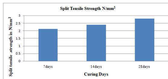
**Figure 4** Graph for Split tensile strength on prism
