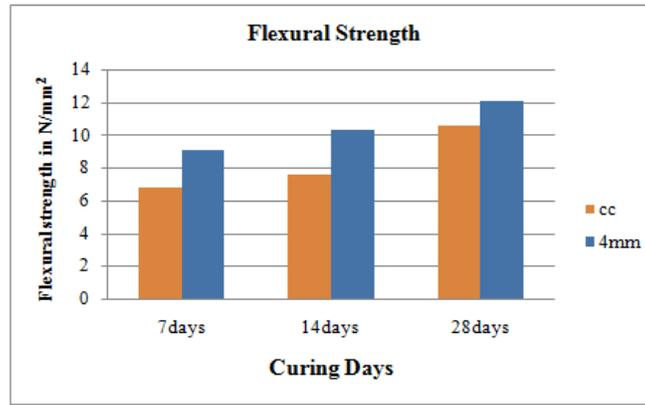
**Figure 7** Graph for CC Vs 4mm thicknesses OC(OPTIMIZED CONCRETE)
