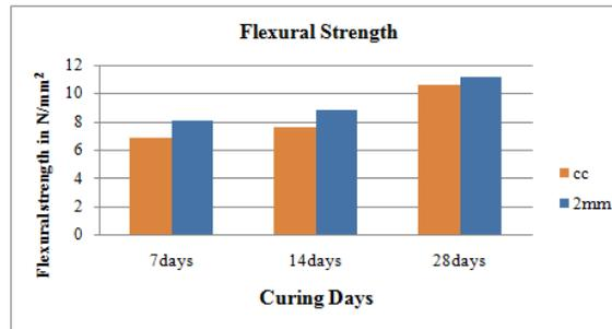
**Figure 5** Graph for CC Vs 2mm thickness OC(OPTIMIZED CONCRETE)
