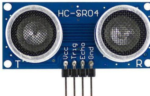
**Figure 3**Ultrasonic Sensor
