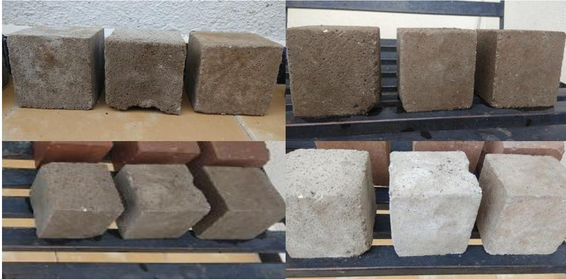
**Figure:5** Samples of stabilized saline sand under the process of wetting and drying
