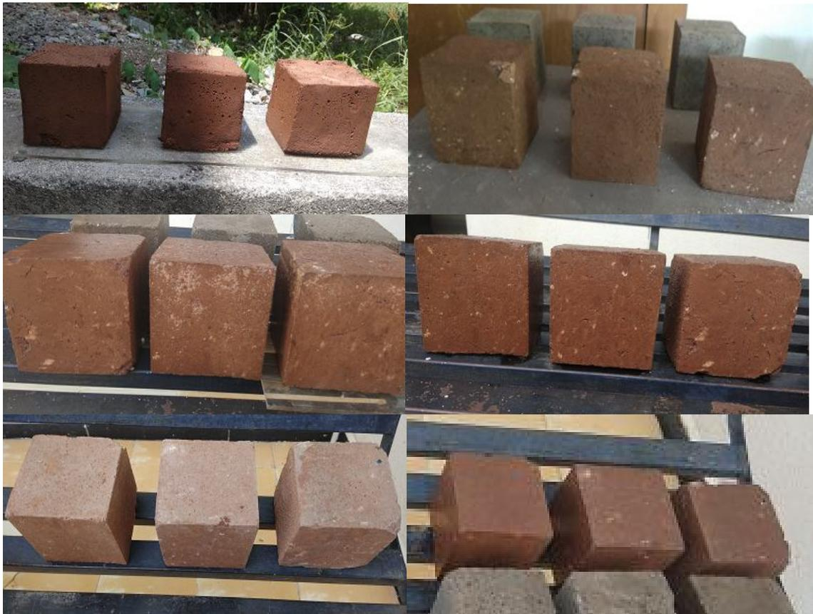
**Figure:4** Samples of stabilized red soil under process of wetting and drying
