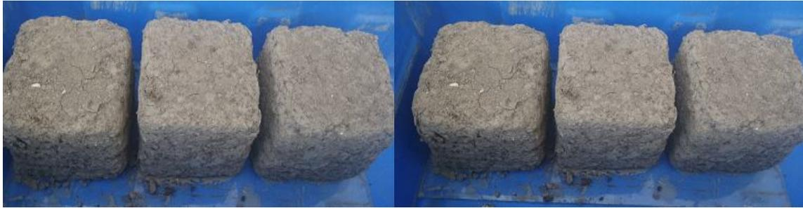
**Figure:3** Samples of black cotton soils after twelfth cycle of drying
