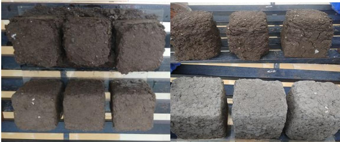
**Figure:2** Samples of Black cotton soil in natural state and stabilized state
