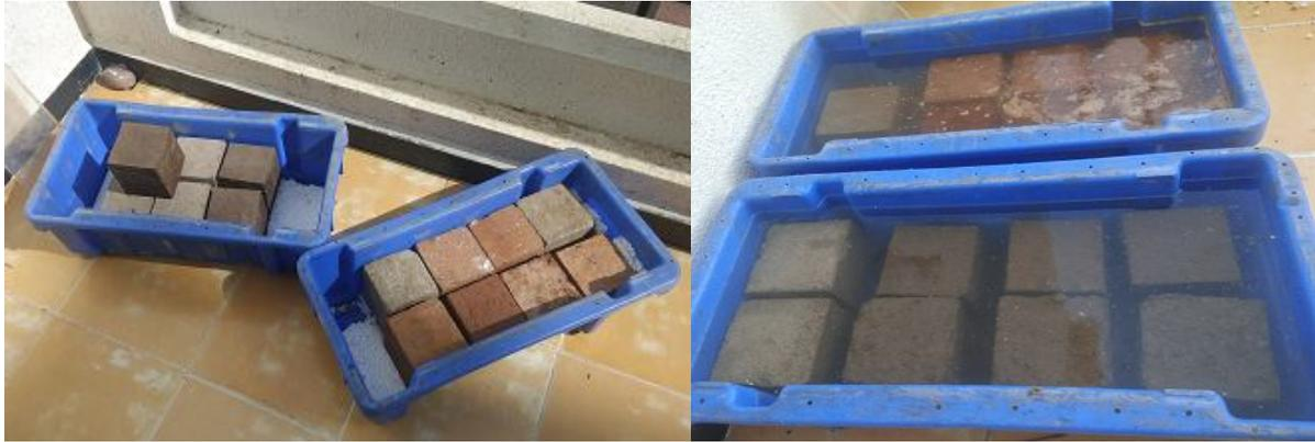
**Figure:1** Wetting and drying process of samples
