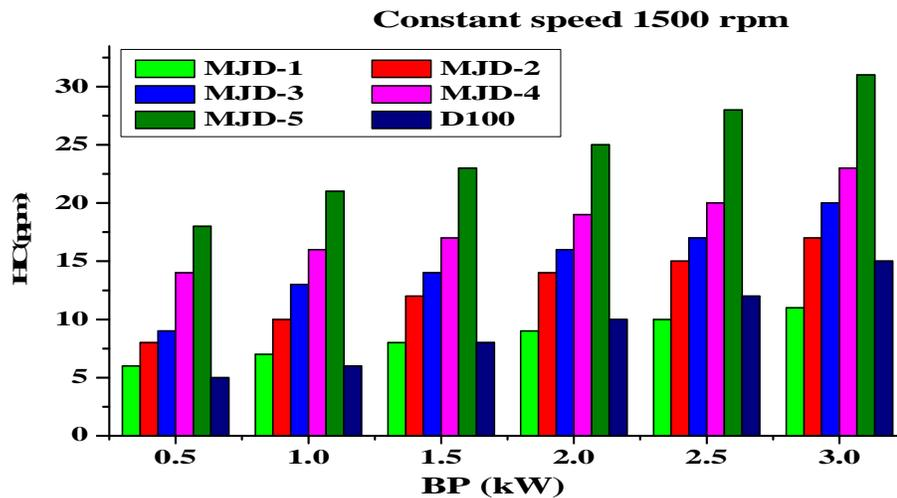
Figure 8. Brake power Vs Hydro carbon emission
