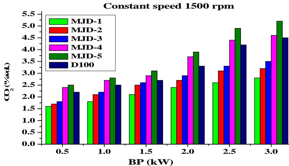
Figure 6. Brake power Vs CO<sub>2</sub> emission
