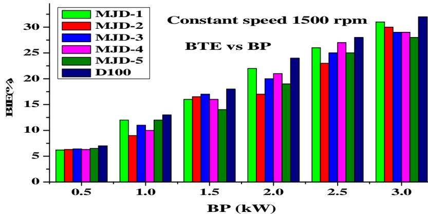
Figure 3. Brake power Vs Brake thermal efficiency
