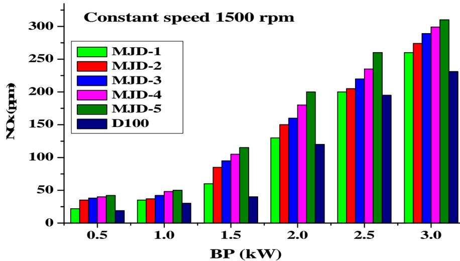
Figure 7. Brake power Vs Nitrogen oxide emission
