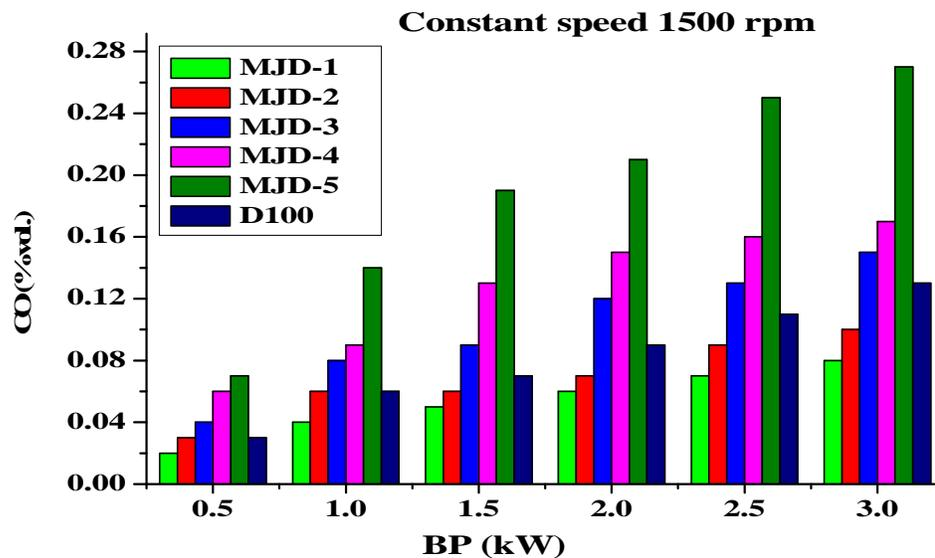
Figure 5. Brake power Vs CO emission
