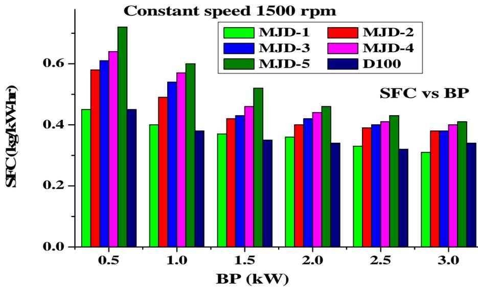
Figure 4. Brake power Vs Specific fuel consumption
