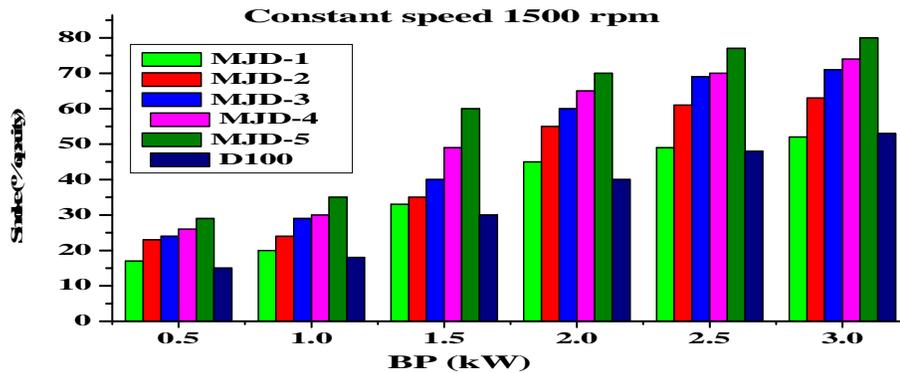
Figure 9. Brake power Vs Smoke emission
